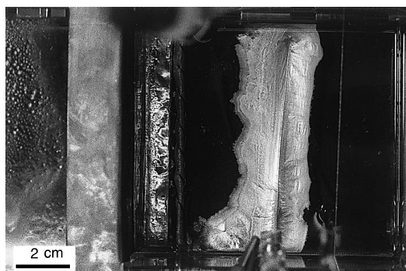
Fig. 7. Growth of a gold film under the rectangular potential electrolysis at -0.2\text{V} for 10 s and at +0.6\text{V} for 20 s for an electrolysis time of 5 h by the line electrode method. Conditions: temperature, 50^\circ\text{C} ; [\text{Na}(\text{AuCl}_4)] , 0.02\text{M} ; [\text{CuSO}_4] , 0.1\text{M} ; [\text{CH}_3\text{COOH}] , 0.1\text{M} ; [\text{CH}_3\text{COONa}] , 0.1\text{M} .
